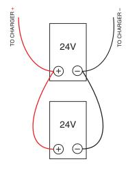
24 VOLT (Parallel Connected) = 24V
